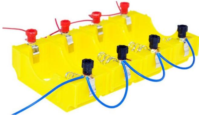
Three series with the battery case, and now the voltage of 4.5V
