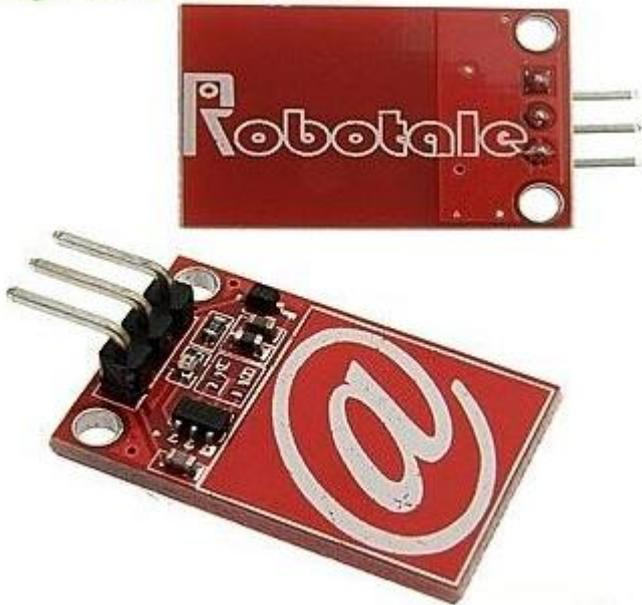
Touch keys detect IC, provide 1 touch keys. Touch detection IC is used to replace the traditional with variable area keys
